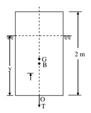
Let the tension in the anchor chain be T kN Total downward force = (W + T) N
