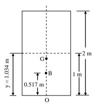
Weight of the buoy = 12 kN = 12000 N
