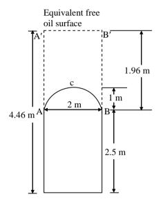
The above figure shows the equivalent free oil surface at a height of 4.46 m above the base of the tank.
