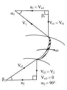
As relative velocity is radial at inlet  $\beta_1$  is 90° As there is no whirl at exit
