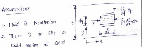
3. Flow is 2-D, steady, Laminor flow.
