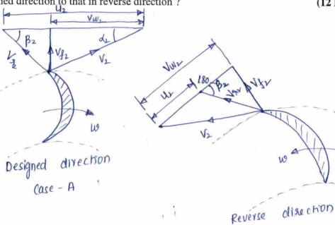
$$(7an \beta_{2}) = \frac{V_{42}}{U_{2} - V_{W2}}$$
