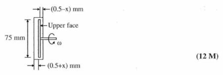
Assume at any point that the velocity profile is linear;
