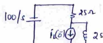
By converting Inductor current and Inductor parallel network into series . it will look like
