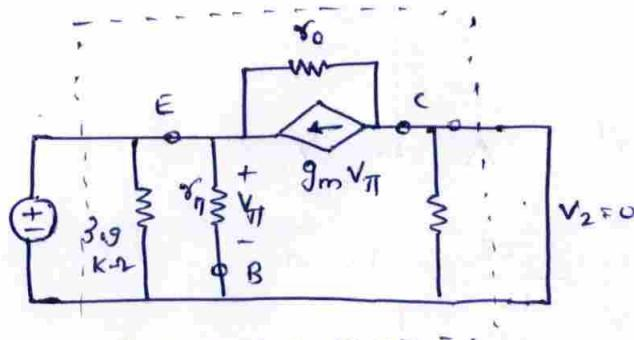
$$\gamma_{\pi} = \frac{B}{g_m} = \frac{100}{3 \text{ mS}} = 33.3 \text{ K}\Omega$$
