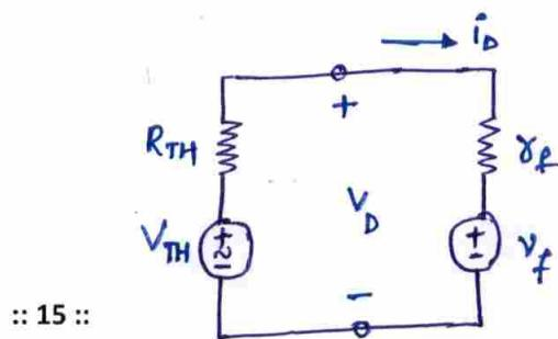
$$V_{TH} = \frac{100}{200} (2 + \cos \omega t) = (1 + 0.5 \cos \omega t) V$$
