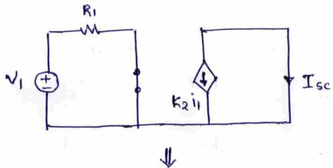
$$\begin{aligned} \dot{i}_1 &= \frac{V_1}{R_1} \\ I_{SC} &= -K_2 \dot{i}_1 \quad \therefore \quad I_{SC} = -\frac{K_2 V_1}{R_1} \end{aligned}$$
