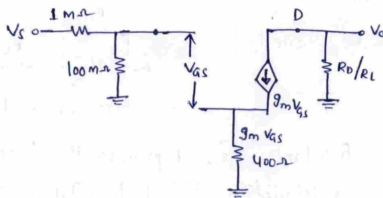
$$V_o = -g_m V_{gs} (R_D / R_L)$$
