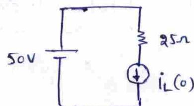
$$\text{Current through Inductor } i_L = \frac{V}{R} = \frac{50}{25} = 2 \text{ A}$$
