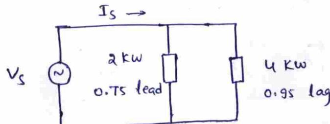
$$P_1 = 2 \text{ kW}, \quad P_2 = 4 \text{ kW}, \quad P_T = 6 \text{ kW}$$
