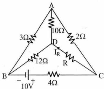
Sol Let current  $I_1, I_2$  and  $I_3$  flow in branches  $AB, AC$  and  $BC$  respectively. Hence current through branches  $AD, CD$  and  $DB$  are  $I_1 - I_2$ ,  $I_2 + I_3$  and  $I_1 + I_3$  respectively.
