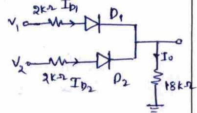
$$\therefore I_{D_1} = I_{D_2}, \quad I_0 = I_{D_1} + I_{D_2} = 4.3 - V_0$$
