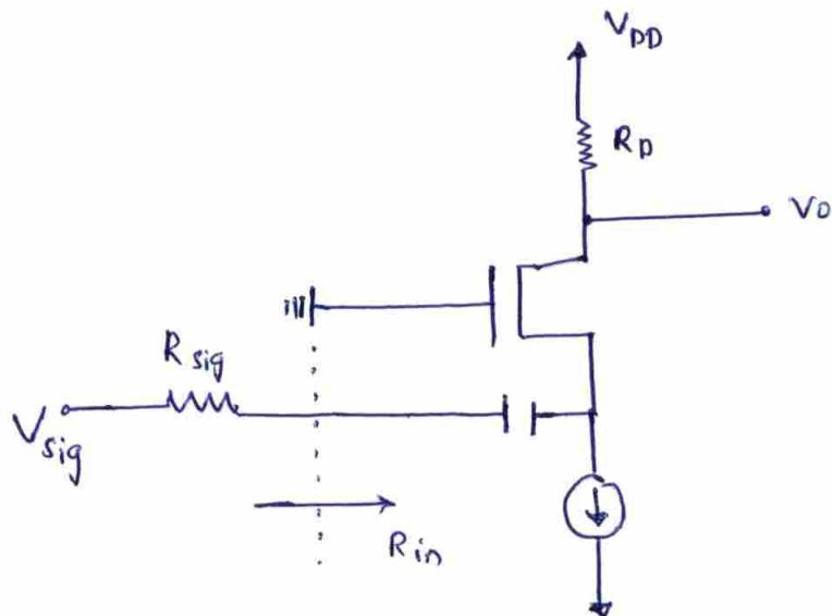
$$R_{\text{in}} = \frac{1}{g_m} = R_{\text{sig}} = 100 \Omega$$
