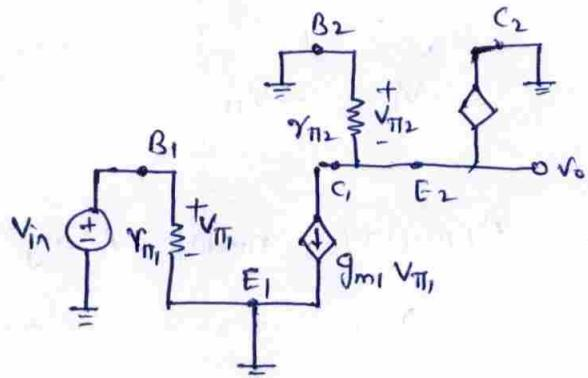
$$g_{m1} \cdot V_{\pi 1} + \frac{V_o}{r_{\pi 2}} = g_{m2} \cdot V_{\pi 2}$$
