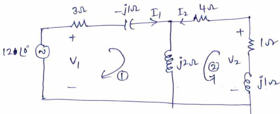
By applying mesh analysis in the above circuit
