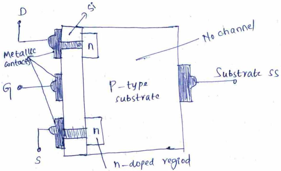
fig(a). Construction of n-channel EMOSFET.
