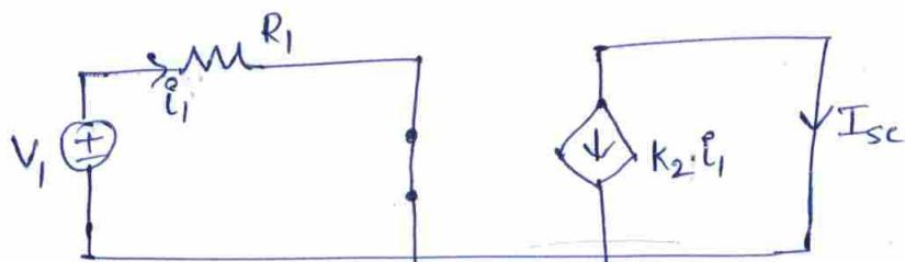
$$i_1 = \frac{V_1}{R_1} ; I_{sc} = -K_2 \cdot i_1$$
