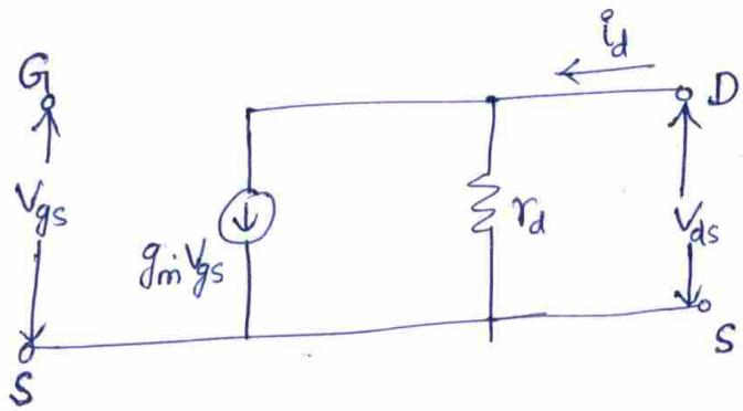
fig : Low frequency small - signal FET Model.
