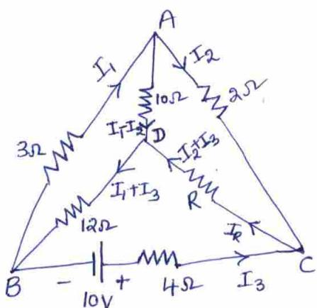
Let current  $I_1$ ,  $I_2$  and  $I_3$  flow in branches AB, AC and BC respectively. Hence, current through branches AD, CD and DB are  $I_1 - I_2$ ,  $I_2 + I_3$  and  $I_1 + I_3$  respectively.
