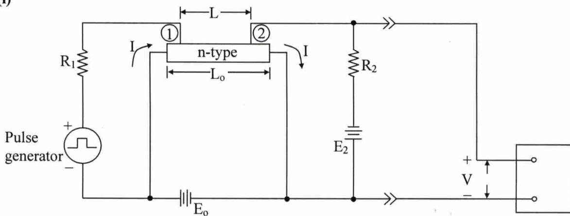
An n-type 'Ge' sample is used in the experiment shown in the above figure. The length of the sample is 1 cm, and the probes (1) and (2) are separated by 0.95 cm. The battery voltage  $E_0$  is 2V. A pulse arrives at point (2) 0.25ms after injection at (1), the width of the pulse  $\Delta t$  is 117  $\mu$ s. Calculate the electron mobility. (8 M)
