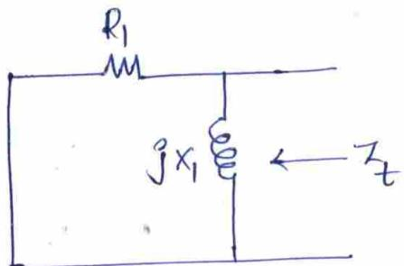
$$Z_t = \frac{R_1(jX_1)}{R_1 + jX_1} = \frac{R_1 X_1^2 + jR_1^2 X_1}{R_1^2 + X_1^2}$$
