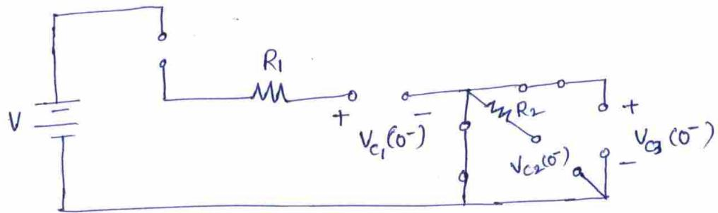
$$\therefore V_{C1}(0^-) = V \text{ Volts}$$
