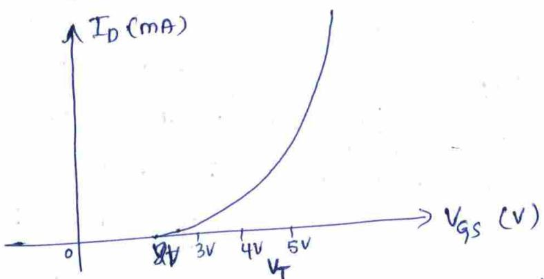
If we increase the magnitude of  $V_{GS}$  in the positive direction, the concentration of electrons near the  $\text{SiO}_2$  surface increases. At a particular value of  $V_{GS}$  there is a measurable current flow between drain and source. This value of  $V_{GS}$  is called Threshold voltage denoted by  $V_T$ .
