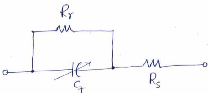
Fig. Circuit model of Varactor diode.
