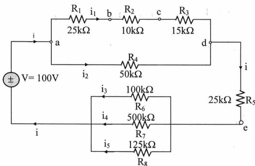
Figure: Series parallel circuit
