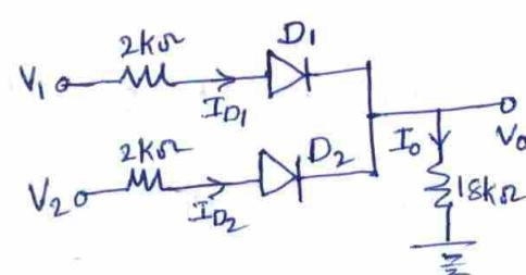
$$\text{Here, } I_{D_1} = \frac{5 - 0.7 - V_0}{2k\Omega} = \frac{(4.3 - V_0)}{2k\Omega}$$
