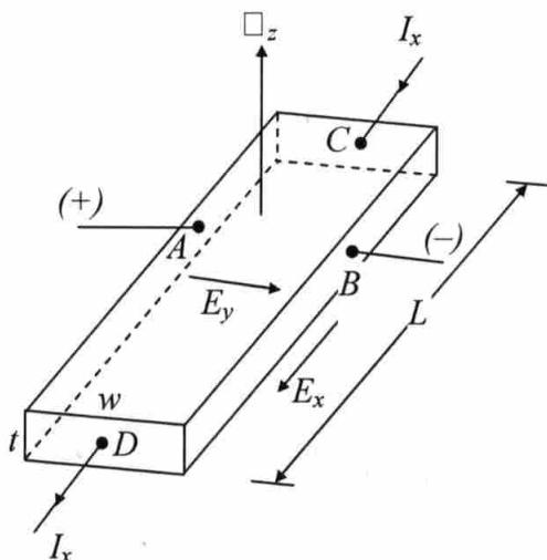
Referring above figure, consider a semiconductor bar with  $W = 0.1\text{mm}$ ,  $t = 10\mu\text{m}$ , and  $L = 5\text{mm}$ . For magnetic flux density,  $B = 10^{-4}\text{wb/cm}^2$  in the direction shown and current of  $1\text{mA}$ , we have  $V_{AB} = -2\text{mV}$  and  $V_{CD} = 100\text{mV}$ . Find the type, concentration and mobility of the majority carrier.
