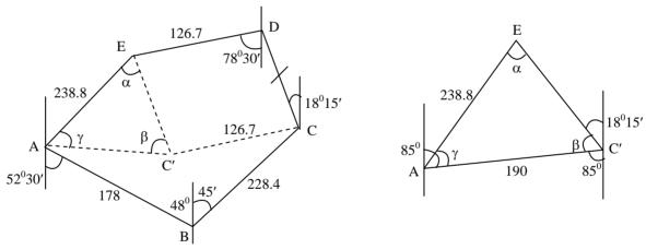
A rough sketch of the traverse is drawn as shown in Fig. above Lines CD and EA are to be brought adjacent. For this, draw a line parallel to CD through E and a line parallel to DE through C. EC' = CD and the two lines with missing measurements are brought adjacent. CC' = DE. The traverse ABCC'A is a closed traverse and the length and bearing of C'A can be found. The calculations are shown in Table below
