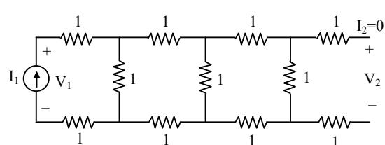
$$Z_{11} = \frac{V_1}{I_1} = [(3 \parallel 1) + 2] \parallel 1 + 2 = 2.73 \Omega$$
