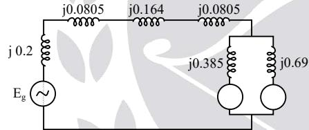
Line reactance =  $\frac{100 \times 25}{(123.2)^2} = 0.164 \text{ pu}$
