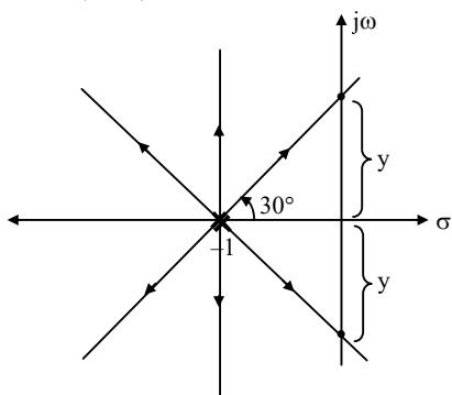
In this case asymptotes become the root locus branches. When 'k' is increased two of the root locus branches move towards  $j\omega$  axis And these two root locus branches cut the  $j\omega$  axis at the point which is obtained as follows
