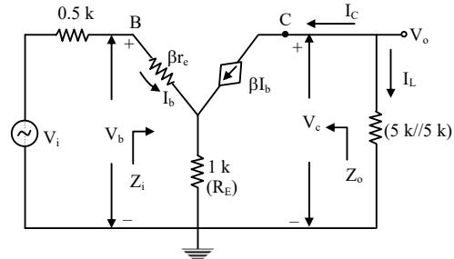
$$A_v = \left( \frac{V_o}{V_b} \right) = \frac{-I_c(2.5k)}{I_b[\beta r_e + (1+\beta)R_E]}$$
