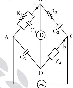
$$\left( \frac{R_1}{1 + j\omega C_1 R_1} \right) Z_4 = \left( R_2 + \frac{1}{j\omega C_2} \right) \frac{1}{j\omega C_3}$$
