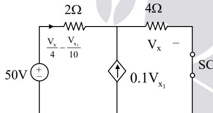
$$50 = \frac{V_{x_1}}{2} - \frac{V_{x_1}}{5} + V_{x_1}$$
