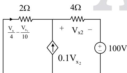
$$\frac{V_{x_2}}{2} - \frac{V_{x_2}}{5} + V_{x_2} + 100 = 0$$
