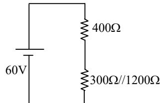
$$R_{eff} = \frac{300\Omega \times 1200\Omega}{1500\Omega} = 240\Omega$$
