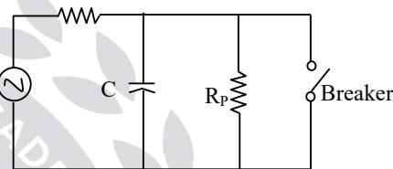
The value of resistance  $R_p$  needed for critical damping of restriking voltage is
