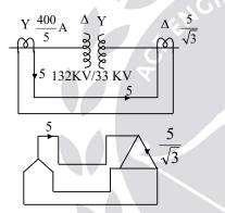
The primary rating of current transformer is obtained by
