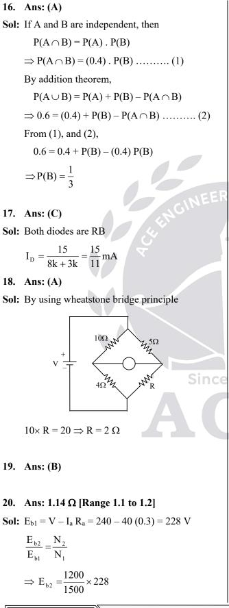
= 182.4 V Now  $E_{b2} = V - I_a (R_a + R_{se}) = 182.4 V$  $\Rightarrow 240 - 40 (0.3 + R_{se}) = 182.4$  $\Rightarrow R_{se} = 1.14 \Omega$
