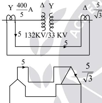
The primary rating of current transformer is obtained by
