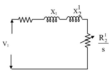
$$\text{For maximum slip, } \frac{R_2^1}{s} = \sqrt{R_1^2 + (X_{01})^2}$$
