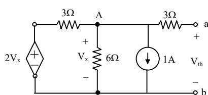
Current flowing through  $3\Omega$  is zero so
