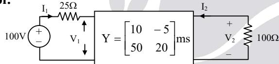
By applying at KVL input side
