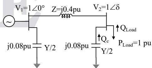
$$P_2 = P_{load} = 1 \text{ pu, as } P_2 = \frac{|V_1||V_2|}{X} \sin(0 - \delta)$$
