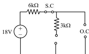
So, L is short circuit, C is open circuit  $i_L(0^-) = 0$
