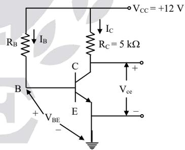
$$V_{CC} = I_B R_B + V_{BE} \dots \dots \dots (1)$$
