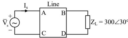
If load is also including in ABCD parameters equivalent ABCD are
