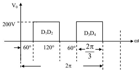
$$\text{Average output voltage, } V_0 = 200 \times \frac{2\pi/3}{\pi}$$
