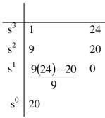
All coefficient of 1<sup>st</sup> row are positive. So, system is stable
