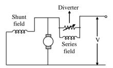
The degree of compounding can be controlled (obtained) by connecting a suitable low resistance across series field winding called "diverter".
