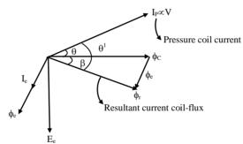
In the above phasor diagram it can be seen that due to eddy currents induced, the phase angle between pressure coil flux and resultant current coil flux is increased.
