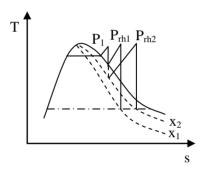
As reheat pressure is lowered, the quality of steam at turbine exhaust increases.
