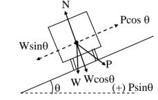
The forces acting on a passenger sitting in a vehicle traversing a horizontal curve of radius 'R' and suprelevation  $\tan \theta$ .
