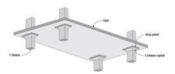
**Flat plate:** It is type of slab supported directly on columns without any stiffening arrangements
