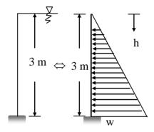
.. If 'h' is depth of water from the top then intensity of load at  $h = \frac{w \times h}{3}$
