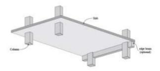
**Ribbed slab:** It is a special type of grid floor, slab – beam system in which the slab is very thin, beams are very slender and are closely spaced.
