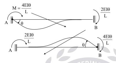
$$\frac{6EI\theta}{L} \underbrace{\frac{6EI\theta}{A}}_{\text{B}} \Rightarrow \theta = \frac{ML}{6EI}$$
