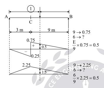
Shear force =  $20 \times 0.5 = 10 \text{ kN}$
