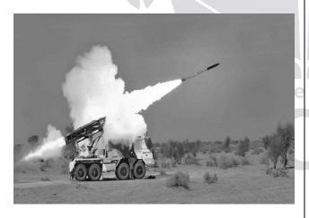
The launcher can fire 12 rockets with 1.2 tonnes of high explosives within 44 seconds and destroy a target area of 4-square km at a time.
