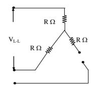
$$P = \frac{(V_{L-L})^2}{(R+R)} = \frac{V_{L-L}^2}{2R}$$
