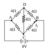
As the bridge is balanced the current flowing through in the branch CD is zero.
