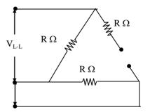
$$P = \frac{(V_{L-L})^2}{R} + \frac{(V_{L-L})^2}{R}$$
