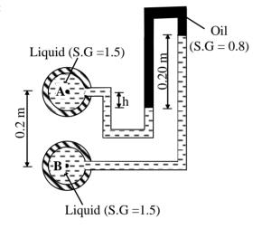
Starting from point A using manometric equation:
