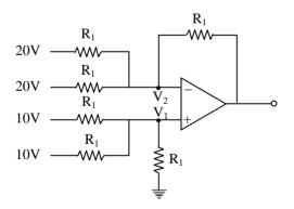
Applying KVL at non inverting node
