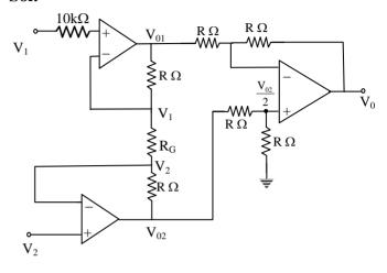
$$\frac{V_2 - V_{02}}{R} + \frac{V_2 - V_1}{R_G} = 0 \qquad (2)$$
