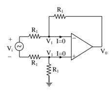
Applying KVL at inverting node
