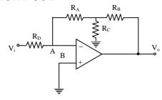
$$Gain = \frac{-\left(R_A + R_B + \frac{R_A R_B}{R_C}\right)}{R_D}$$
