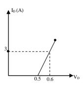
$$P_{D} = V_{D}I_{D} + I_{D}^{2}r_{DC}$$
