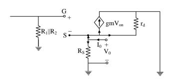
$$\begin{split} V_{GS} &= -V_0 \\ I_0 &= \frac{V_0}{R_s} + \frac{V_0}{r_d} + g_m V_{GS} \\ &= V_0 \Bigg[ \frac{1}{R_s} + \frac{1}{r_d} + g_m \Bigg] \\ \frac{V_0}{I_0} &= \frac{1}{\frac{1}{R_s} + \frac{1}{r_d} + \frac{1}{1/g_m}} \\ &= R_s \parallel r_d \parallel 1/g_m \\ &= 2k \parallel 1/1m \\ &= \frac{2 \times 1}{2 + 1} = \frac{2}{3}k \end{split}$$
