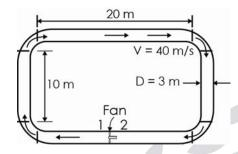
Applying Energy equation for two points, just upstream and downstream of the fan in the pipe loop.
