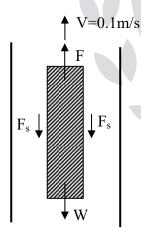
The thickness of the oil layer is same on either side of plate
