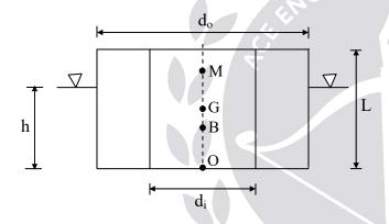
Let 'h' be the depth of immersion of the cylinder in oil and L be the height of the cylinder.
