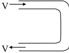
$$\begin{aligned} F_x &= \rho aV( V_{1x} - V_{2x}) \\ &= \rho aV( V - (-V)) \\ &= 2 \rho a V^2 \\ &= 2 \times 1000 \times 10^{-4} \times 5^2 = 5 \text{ N} \end{aligned}$$
