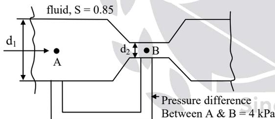
$$d_1 = 300 \text{ mm}, \quad d_2 = 120 \text{ mm}$$
