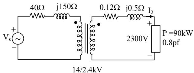
The equivalent circuit refer to L.V side is
