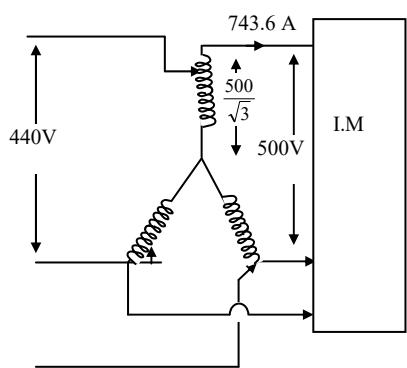
$$I_2 = \frac{610 \times 0.745 \times 10^3}{\sqrt{3} \times 500 \times 0.8 \times 0.882} \\ = 743.69 \text{ A}$$
