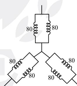
$$E_{ph} = 4.44 \times 0.951 \times 0.957 \times 0.025 \times 50 \times 80 \\ = 404 V$$
