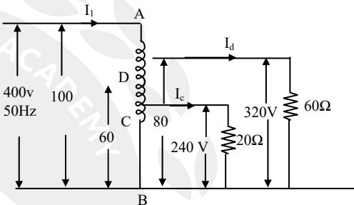
$$\text{The voltage per turn} = \frac{400}{100} = 4 \text{ V}$$
