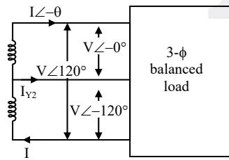
$I_{Y2}$  is  $-120^\circ$  lagging w.r.t  $I \angle -\theta$  (from 3φ system)
