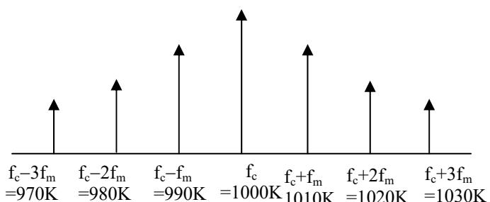
These frequencies 980K, 1020K are not present because the symmetrical square wave it consists of half wave symmetries only odd harmonics are present, even harmonics are dismissed
