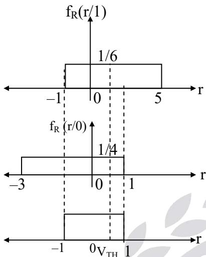
For minimum error the  $V_{TH}$  should lie in the area of intersection of the 2 pdf's.
