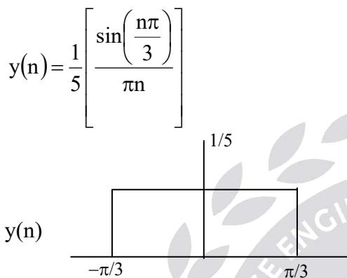
$$\sum_{n=-\infty}^{\infty} \frac{\sin \frac{n\pi}{4}}{2\pi n} \times \frac{\sin \frac{n\pi}{3}}{5\pi n} = \frac{1}{2\pi} \int_{-\frac{\pi}{4}}^{\frac{\pi}{4}} \left( \frac{1}{2} \right) \left( \frac{1}{5} \right) d\omega$$
