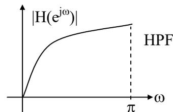
And it is FIR Filter because finite coefficients
