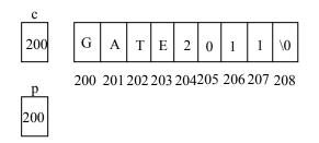
ASCII value of A = 65 ASCII value of C = 69 printf ("%s", p + p[3] - p[1]) printf("%s", 200 + 69 - 65) printf("%s", 204) Output = 2011
