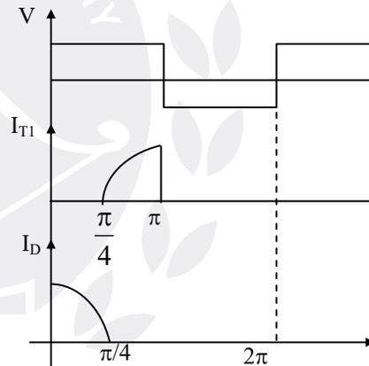
$$(i_T)_{RMS}^2 = \frac{1}{2\pi} \int_{\pi/4}^{\pi} I_m^2 \sin^2 \omega t d(\omega t)$$
