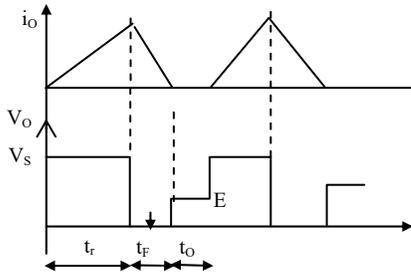
From above diagram  $t = t_r + t_f + t_o$
