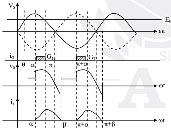
When  $T_1 T_2$  pair is ON at  $\omega t = \alpha$
