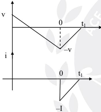
$$(E_{\text{loss}})_{\text{OFF}} = \int_0^{t_1} v i dt$$
