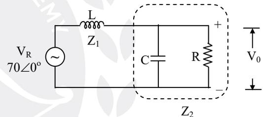
$$V_0 = 70 \angle 0^\circ \times \frac{Z_2}{Z_1 + Z_2}$$
