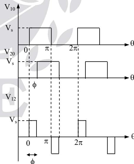
Explanation: At instant 0,  $V_{10} = V_s$  and  $V_{20} = 0$
