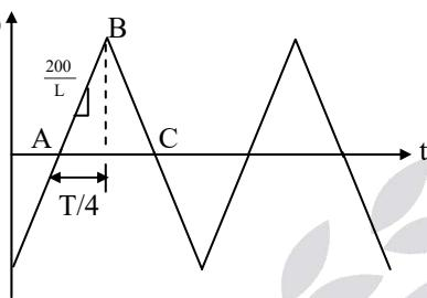
$$y = mx, I_p = \frac{200}{L} \times \frac{T}{4} \quad [T = 20 \text{ msec}]$$
