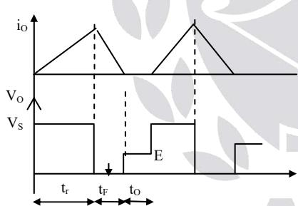
From above diagram  $t = t_r + t_f + t_o$
