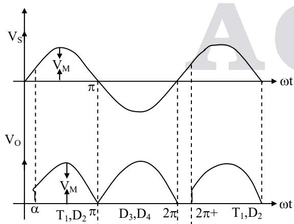
During positive half cycle  $T_1$  and  $D_2$  are forward biased
