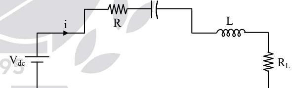
$$\text{KVL} \quad V_{\text{dc}} = (R + R_L) i + L \frac{di}{dt}$$
