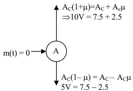
$$\text{Amplitude deviation } A_C\mu = 7.5 \times \frac{1}{3} = 2.5 \text{ V}$$
