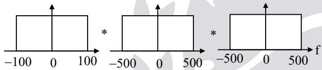
So, highest frequency component in the signal  $m(t)$  is  $100 + 500 + 500 = 1100$
