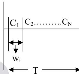
$$\text{Minimum B.W of TDM is } \sum_{i=1}^N w_i$$
