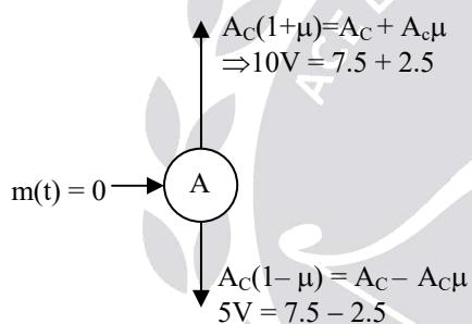
$$\text{Amplitude deviation } A_C\mu = 7.5 \times \frac{1}{3} = 2.5 V$$
