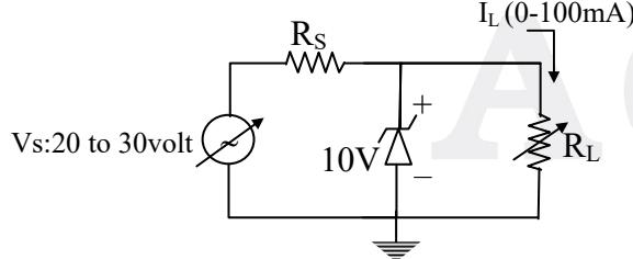
The current in the diode is minimum when the load current is maximum and  $v_s$  is minimum.
