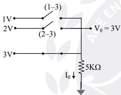
⇒ D<sub>1</sub>, D<sub>2</sub> are reverse biased and D<sub>3</sub> is forward biased.
