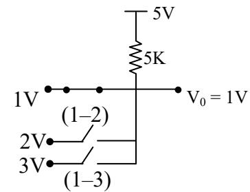
⇒ D<sub>2</sub> & D<sub>3</sub> are reverse biased and 'D<sub>1</sub>' is forward biased.
