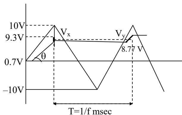
When diode is OFF, the capacitor discharges through the resistor
