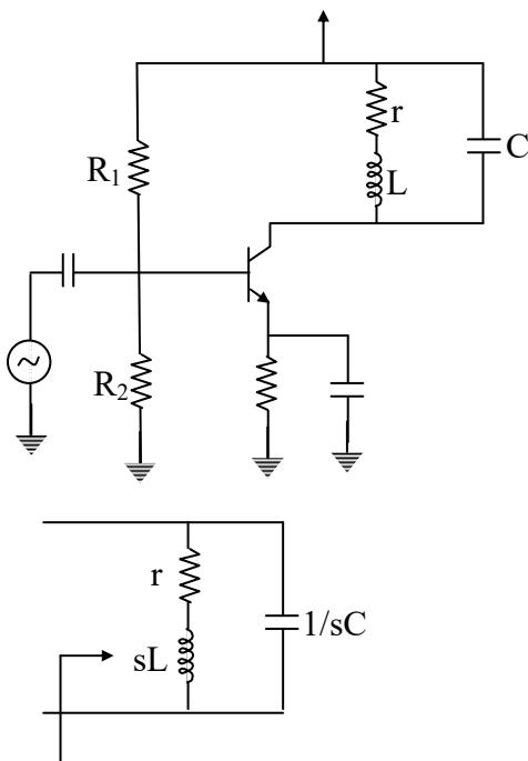
$$\begin{aligned} Z_{eq} &= \frac{1}{sC + \frac{1}{r+sL}} \\ &= \frac{r+sL}{srC + s^2LC + 1} \\ &= \frac{r+j\omega L}{(1-\omega^2LC) + j\omega rC} \\ Z_{eq} &= \frac{(r+j\omega L)[1-\omega^2LC - j\omega rC]}{(1-\omega^2LC)^2 + (\omega rC)^2} \end{aligned}$$
