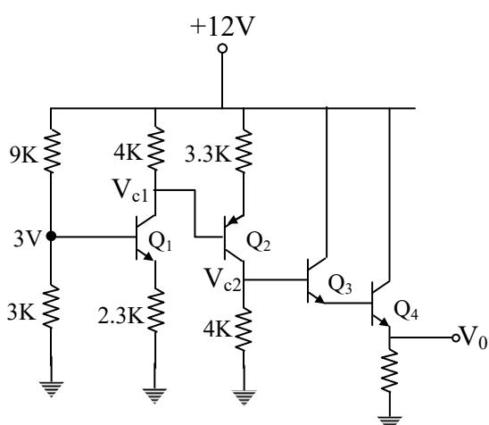
$$I_{C_1} = I_{e_1} = \frac{2.3V}{2.3k} = 1 \text{ mA}$$
