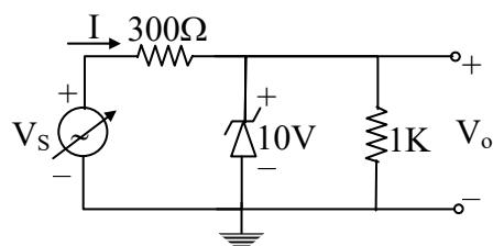
$$I_z = 1\text{mA} \text{ to } 60\text{mA}$$
