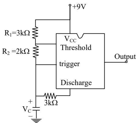
$$V_{th} = \frac{2}{3} V_{CC} = \frac{2}{3} \times 9 = 6 \text{ V}$$
