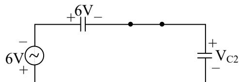
$$V_{C_2} = -6 - 6 = -12V$$
