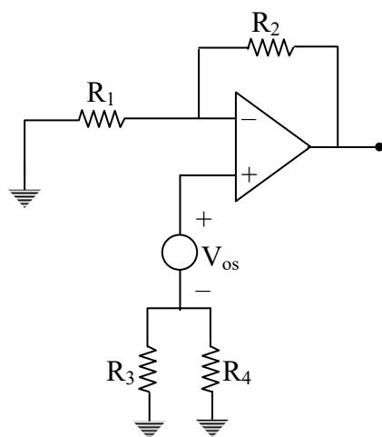
$$\begin{aligned}V_0 &= \left[1 + \frac{R_2}{R_1}\right]V_{os} + I_{os}R_2 \\&= \left[1 + \frac{1M}{10k}\right]4mV + 50nA[1M] \\&= 454mV\end{aligned}$$
