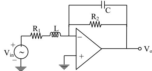
$$Z_2 = R_2 \parallel \frac{1}{sC} = \frac{R_2}{sCR_2 + 1}$$
