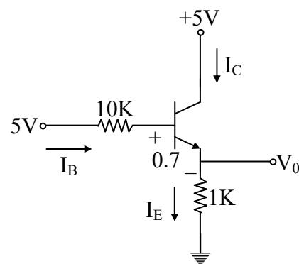
Apply KVL to the base emitter loop:
