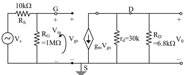
$$V_0 = -g_m V_{gs} (r_d || R_D)$$
