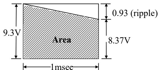
$$(a) V_{Avg} = \frac{\text{Area}}{\text{Base}} = \frac{9.3(1m) - \frac{1}{2}(0.93)(1m)}{1m} \\ = 9.3 - \frac{0.93}{2} = 8.84V$$
