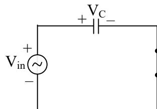
$$V_{C_1} = V_{in} = 6\text{ volt}$$
