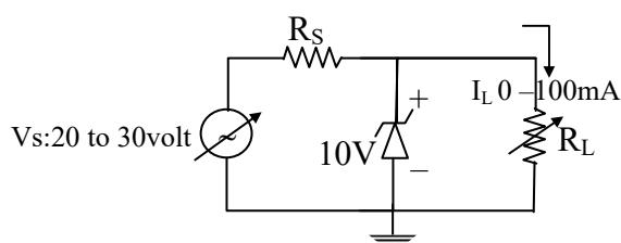
The current in the diode is minimum when the load current is maximum and  $v_s$  is minimum.
