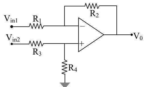
$$\begin{aligned} V_0 &= \frac{R_2}{R_1} (V_{in2} - V_{in1}) \\ &= \frac{1M}{10k} (V_{in2} - V_{in1}) \end{aligned}$$
