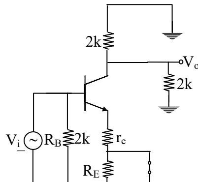
$$A_v = \frac{V_0}{V_i} = \frac{-R_C}{r_e} = \frac{-(2k \parallel 2k)}{25.22} = -39.65$$
