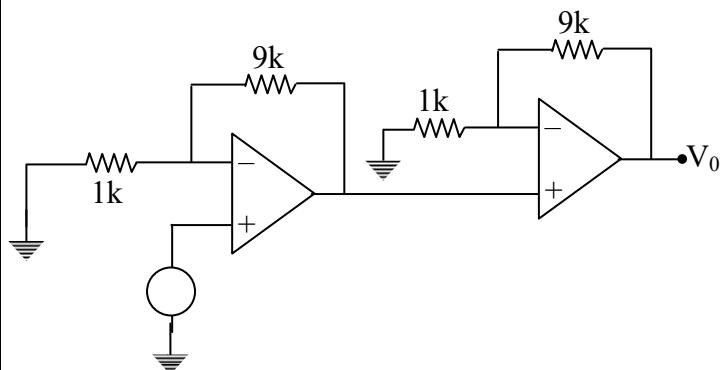
$$\begin{aligned} \text{Overall BW} &= f_{3dB} \sqrt{2^{1/2} - 1} \\ &= 100\text{k} (0.04) \\ &= 64\text{ kHz} \end{aligned}$$
