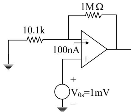
$$\begin{aligned} V_0 &= |V_{0_{\text{Bias current}}}| + |V_{0_{\text{Offset Voltage}}}| \\ &= 1M(I_B) + \left(1 + \frac{R_2}{R_1}\right)V_{os} \\ &= 1M(100nA) + 100(1mV) \\ &= 0.2V \end{aligned}$$
