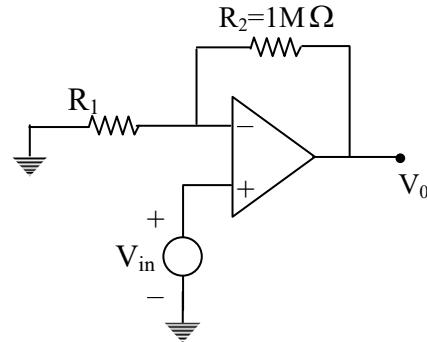
$$\text{Gain} = \frac{V_o}{V_{in}} = 1 + \frac{1M}{R_1} = 100 \Rightarrow R_1 = 10.1\text{k}\Omega$$
