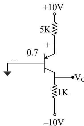
$$V_E = 0.7\text{V} [\because V_B = 0\text{V}]$$
