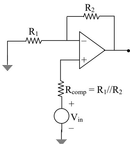
$$\begin{aligned} \rightarrow R_{\text{comp}} &= R_1//R_2, \text{ then } V_0 = (I_{B1} - I_{B2}) R_2 \\ &= I_{os} R_2 \\ V_0 &= (I_{B1} - I_{B2}) R_2 \\ &= I_{os} R_2 \\ &= 1/10 (I_B R_2) \end{aligned}$$
