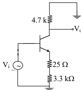
$$\frac{V_0}{V_i} = \frac{-R_c}{r_e + R_E} = \frac{-4700}{25 + 3300}$$
