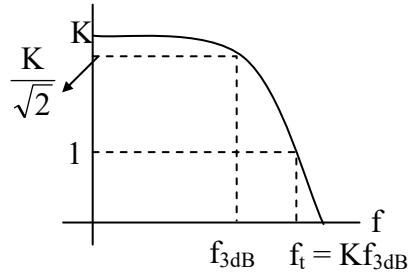
(b) Gain = 40dB = 100,  $f_t = 1\text{MHz} = \text{Gain BW}$
