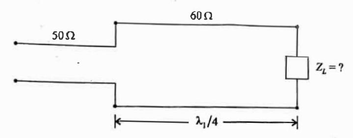
Find the load impedance which can be matched to a 50  $\Omega$  transmission line with a quarter wave line (at  $\int = f_1$ ) of characteristic impedance 60  $\Omega$ . If the frequency is doubled (at  $f = 2f_1$ ), what will be the VSWR on 50  $\Omega$  line? 20
