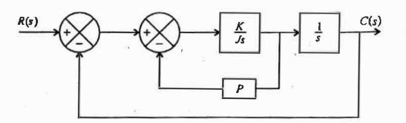
Determine the value of K & P of the closed loop system shown in the figure, so that the maximum overshoot in unit step response is 25% and the peak time is 2 sec. Assume that  $J = 1 \text{ kg-m}^2$ . 10
