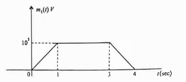
Consider a message signal  $m_1(t)$  as shown and message signal  $m_2(t) = \sin c (2 \times 10^4 t)$ , in volts.
