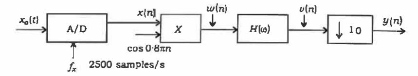
In this system,  $H(\omega)$  is a low-pass filter with a discrete cut-off frequency equivalent to  $f_c = 125$  Hz (normalized w.r.t. the sample rate at the point in the block diagram). Determine and sketch the spectra of  $X(\omega_x)$ ,  $W(\omega_w)$ ,  $V(\omega_w)$  and  $Y(\omega_y)$  w.r.t.  $\omega_x$ ,  $\omega_w$ ,  $\omega_v$  and  $\omega_y$  respectively for  $-\pi < \omega < \pi$ . 20
