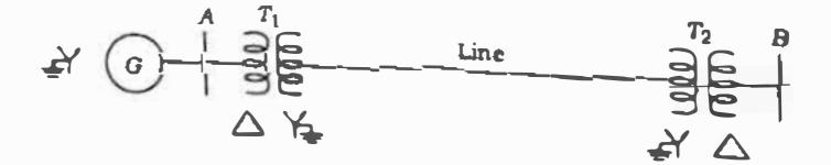
The ratings of the equipments are the following : Generator G: 15 MVA, 6.6 kV,  $X_1 = 15\%$ ,  $X_2 = 10\%$ Transformers: 15 MVA, 6.6 kV delta/33 kV star,  $X_1 = X_2 = X_0 = 6\%$ Line reactance :  $X_1 = X_2 = 2\Omega$  and  $X_0 = 6\Omega$ Find the fault current for a ground fault on one of the bus bars at B. 20
