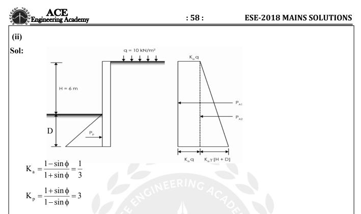
Approximate analysis is used to determine depth of embedment of sheet pile wall. In the approximate analysis, the active earth pressure on the back of the wall and the passive earth pressure infront of the wall are assumed to extend upto base of the wall as shown in figure.
