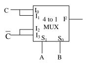
$F = \overline{A}\overline{B}C + \overline{A}BC + A\overline{B}\overline{C} + AB\overline{C}$  $F = \overline{A}C(B + \overline{B}) + A\overline{C}(B + \overline{B})$  $F = \overline{A}C + A\overline{C} = A \oplus C$
