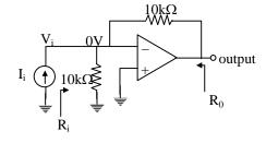
Input resistance (R<sub>i</sub>) =  $\frac{V_i}{I_i} = \frac{0}{0.5m} = 0\Omega$
