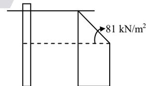
$$\text{Critical depth} = 15 \times \text{diameter}$$
