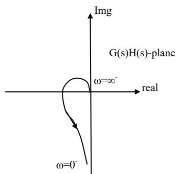
**Mapping of section C<sub>4</sub>:** It is the radius 'ε' semicircle, therefore  $\text{sub } s = \lim_{\varepsilon \rightarrow 0} \varepsilon e^{j\theta}$  ( $-90^\circ \leq \theta \leq 90^\circ$ ) in the TF  $G(s)H(s)$ , which gives clockwise infinite radius semicircle in  $G(s)H(s)$  plane.
