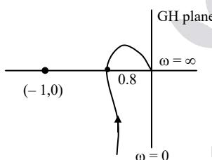
even though the value of  $K$  is double, the system is stable (negative real axis magnitude is less than one)
