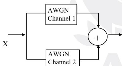
At the input of the receiver signal amplitude is doubled. But when two independent Gaussian Random Variables are added, the resultant random variables is also a Gaussian random. The pdf is the convolution of individual pdf's. The variance indicates the noise power
