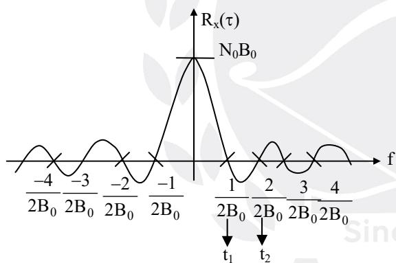
$$|t_1 - t_2| = \text{multiple of } \frac{1}{2B}$$
