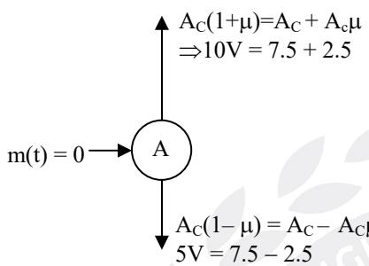
$$\text{Amplitude deviation } A_c\mu = 7.5 \times \frac{1}{3} = 2.5 \text{ V}$$
