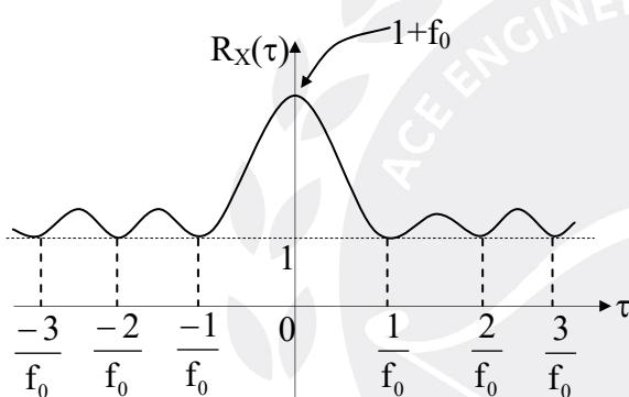
(b) Since  $R_X(\tau)$  contains a constant component of amplitude 1. It follows that the dc power contained in  $X(t)$  is 1.
