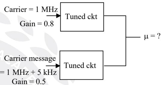
$$\begin{aligned} S(t) &= 0.8 \times 10\cos 2\pi 10^6 t \\ &\quad + 0.5 \times 8\cos 2\pi 5000 t \cos 2\pi 10^6 t \\ &= 8\left(1 + \frac{4}{8}\cos 2\pi 5000 t\right) \cos 2\pi 10^6 t \end{aligned}$$
