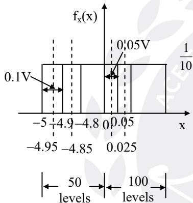
$$\text{Signal power } E[X^2] = \int_{-5}^5 x^2 \left(\frac{1}{10}\right) dx \\ = \frac{1}{10} \left(\frac{x^3}{3}\right)_{-5}^5 = \frac{1}{30}(250) = \frac{25}{3} \text{ W}$$
