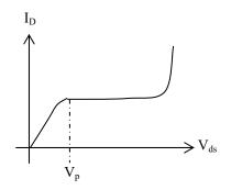
Drain current remains constant at pinch off region even if the drain voltage increases.
