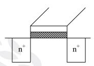
$$\begin{split} A &= (0.2\mu \times 1\mu) + (0.2\mu \times 1\mu) + (0.2\mu \times 1\mu) \\ &= 3(0.2\mu \times 1\mu) = 0.6 \times 10^{-12} \text{ m}^2 \\ C_{sbo} &= \frac{11.7 \times 8.9 \times 10^{-12} \times 0.6 \times 10^{-12}}{10 \times 10^{-9}} \\ C_{sbo} &= 6.24 \times 10^{-15} \end{split}$$
