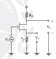
$$\frac{V_2}{V_i} = \frac{g_m R_s}{1 + g_m R_s}$$
