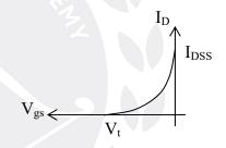
$$\begin{aligned} V_{gs} &= V_t & I_D &= 0 \\ V_{gs} &= 0 & I_D &= I_{DSS} \end{aligned}$$
