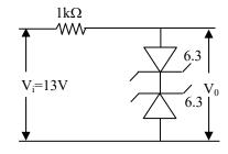
$$V_0 = 0.6 + 6.3 = 6.9 \text{ V}$$
