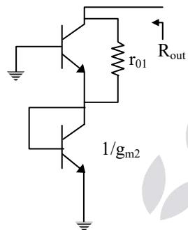
$$\begin{aligned} R_{out} &= r_{01} + (1+g_{m1} r_{01}) \frac{1}{g_{m2}} \\ &= r_{01} + \frac{1}{g_{m2}} + r_{01} \\ &= 2 r_{01} \end{aligned}$$
