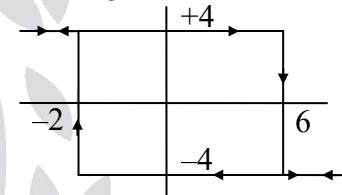
$$\text{Hysteresis width} = \text{UTP} - \text{LTP} \\ = 6 - (-2) = 8\text{V}$$
