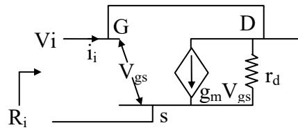
$$R_i = \frac{V_i}{i_i}, \text{ where } i_i = g_m V_{gs} + \frac{V_i}{r_d}$$
