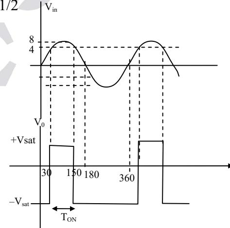
$$T_{ON} = 120^\circ, T = 360^\circ$$
