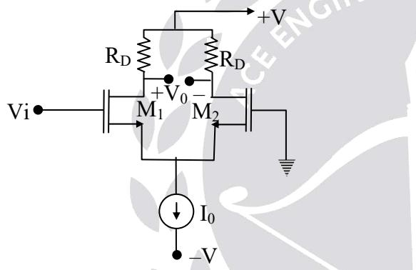
$$\text{For } M_1 \rightarrow V_{01}. \text{gain} = -g_{m_1} \frac{R_o}{2} \Rightarrow g_{m_1} \frac{R_o}{2} V_i$$
