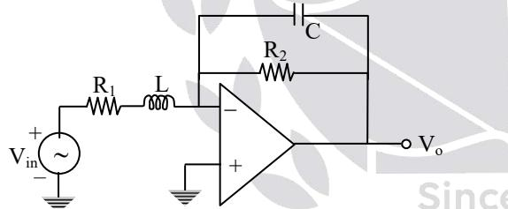
$$z_2 = R_2 \parallel \frac{1}{sC} = \frac{R_2}{sCR_2 + 1}$$
