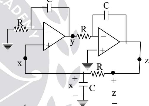
$$\frac{y}{x} = 1 + \frac{sC}{R} = 1 + \frac{1}{sCR} = \frac{sCR + 1}{sCR} \dots\dots(1)$$
