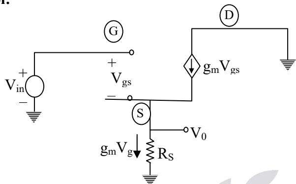
$$V_o = g_m V_{gs} R_s$$
