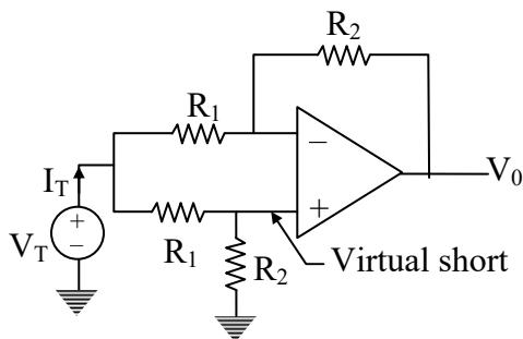
Due to virtual short Two  $R_1$  resistors are looking as in parallel
