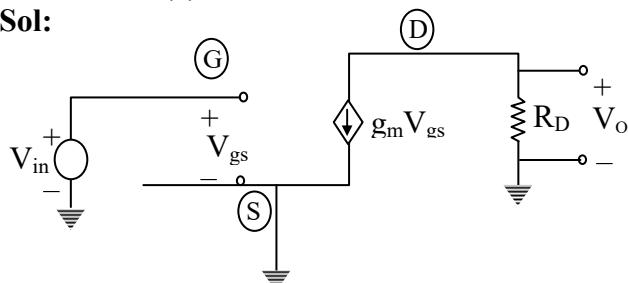
$$\left. \begin{aligned} V_o &= -g_m V_{gs} R_D \\ V_{in} &= V_{gs} \end{aligned} \right\} \frac{V_o}{V_{in}} = -g_m R_D$$
