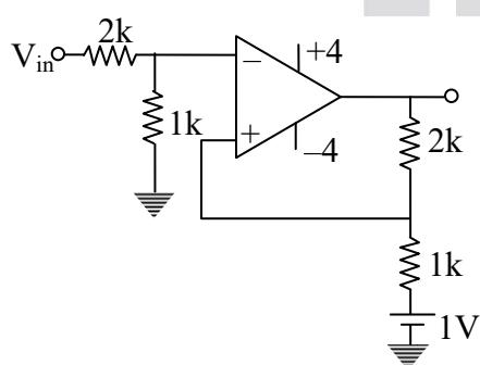
$$V_- = \frac{V_{in} \times 1}{1 + 2} = \frac{V_{in}}{3}$$
