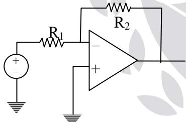
$$V_0 = -\frac{R_2}{R_1} \times V_{in}$$
