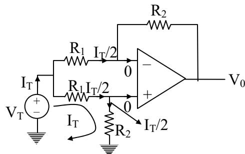
$$\text{Writing KVL; } V_T = \frac{I_T}{2} \times R_1 + \frac{I_T}{2} \times R_2 \\ = \frac{I_T}{2} (R_1 + R_2)$$
