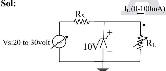
The current in the diode is minimum when the load current is maximum and  $v_s$  is minimum.
