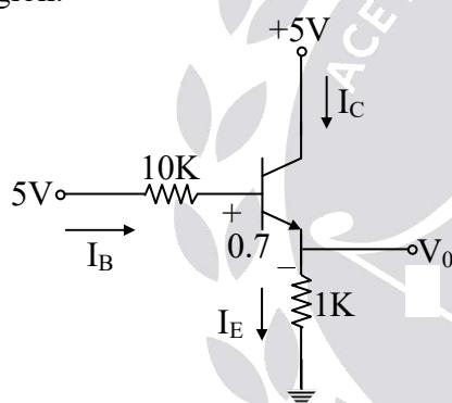
Apply KVL to the base emitter loop:
