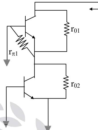
$$R_{out} = r_{01} + (+g_m r_{01}) \\ (r_{02}/r_{\pi 2}) \\ = r_{01} + r_{\pi 2} + g_m r_{01} r_{\pi 2} \\ = r_{01} + \beta r_{01} \\ = (\beta + 1) r_{01} \\ \approx \beta r_{01}$$
