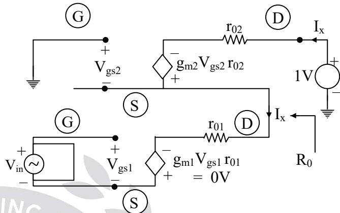
$$\text{By KVL } V_{gs2} + I_x r_{01} = 0$$
