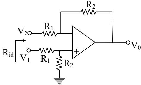
To find input resistance  $R_{id}$  (differential input resistance) look from input port.
