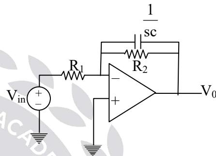
$$\frac{R_2 \times \frac{1}{sc}}{R_2 + \frac{1}{sc}} = \frac{R_2}{1 + scR_2} = Z_2 \dots\dots(1)$$
