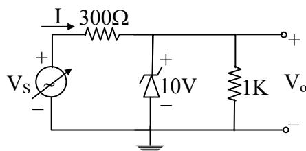
$$I_z = 1\text{mA} \text{ to } 60\text{mA}$$
